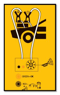
3. If the unit is 'activated' then the light shows red and the buzzer sounds. Once the unit has been activated it is rendered useless for future use and must be replaced.
