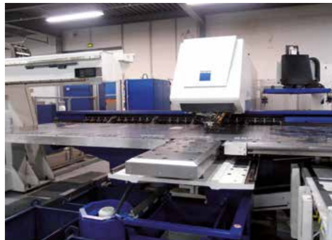
The robotic machines take metal plates and place them into the correct working position where oval vents, oblong mouldings, square or round holes are cut. Each piece is bespoke for the application.
