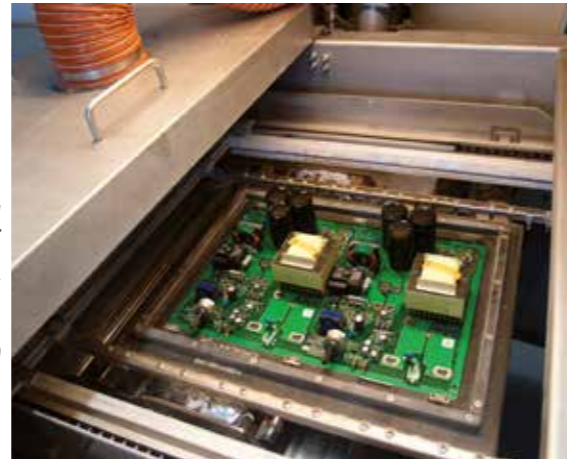
New welding robot for electronic cards. The card is immersed in a bath which can weld its 200 components in a single process.
