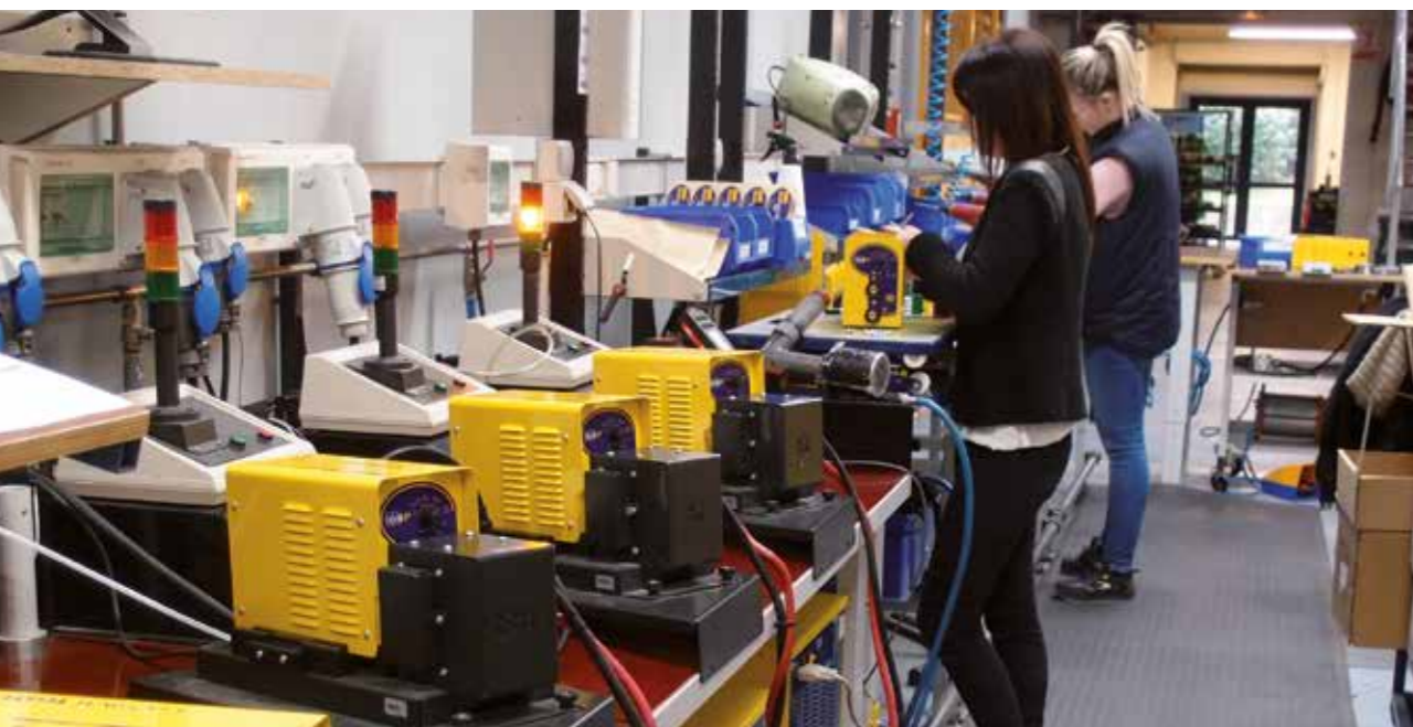
For complete traceability, all tests are recorded in real time during the final test. The user has access to the entire product's path through the 2D bar code printed on the machine.
