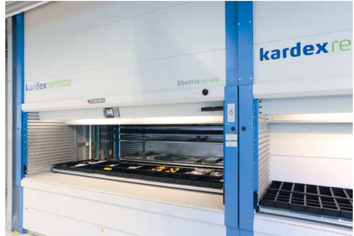
The company has invested in a Kardex storage system for the electronic cards' components. Eleven million components are stored on two levels.
