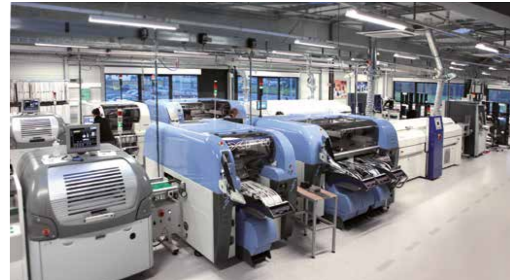
The assembly of electronic cards is fully automated.
