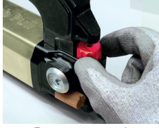
Pressure control 0 > 6.5 bar
