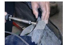
Do not press too hard on the soldering iron. The temperature of 550°C of the tip is quite sufficient to make the melted plastic go back up through the stainless steel mesh. Once this operation has been performed, and for a very limited cost, your bumper already has quite a good resistance to stress and shocks (photo 2).
