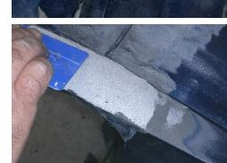
In this case, after perfectly sanding and removing grease on the edge of the break, braze with the JBDC brazing sticks.
